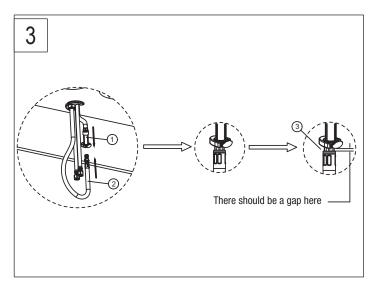
3. Connect the outlet hose (1) with pull-down hose (2). Confirm the bushing (3) return to original state.
