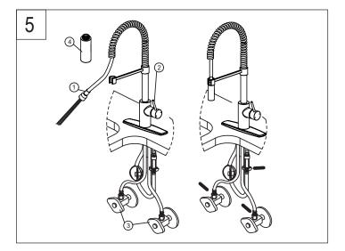
5. Connect to water supplies (hot and cold angle valve).
