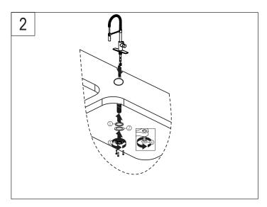
2. Thread the faucet through the mounting hole. Secure to sink by rubber washer (1), steel washer (2), tighten the lock nut (3), and mounting screws (4). Do not over tighten.
